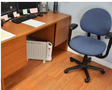
Heater misuse hazard
